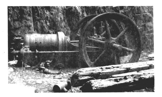
The gas engine was made in Gloucester by Fielding & Platt Ltd. It has a single, horizontal cylinder, mounted on a cast-iron bed, which is bolted to a masonry plinth. Twin flywheels, and a flat belt-drive pulley, are carried on the open crankshaft. The engine was fuelled by gas made in a vertical cylindrical gas generator plumbed directly into the engine. The sawing frame, an iron and wood structure about 12 feet high, was made in Arbroath.
