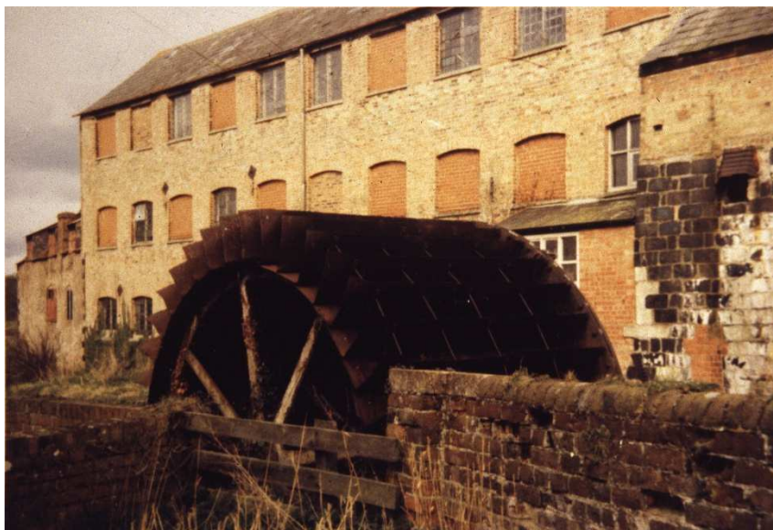
Picture 2 The wheel's opposite side. The second (inner) wheel was later replaced by a water turbine
