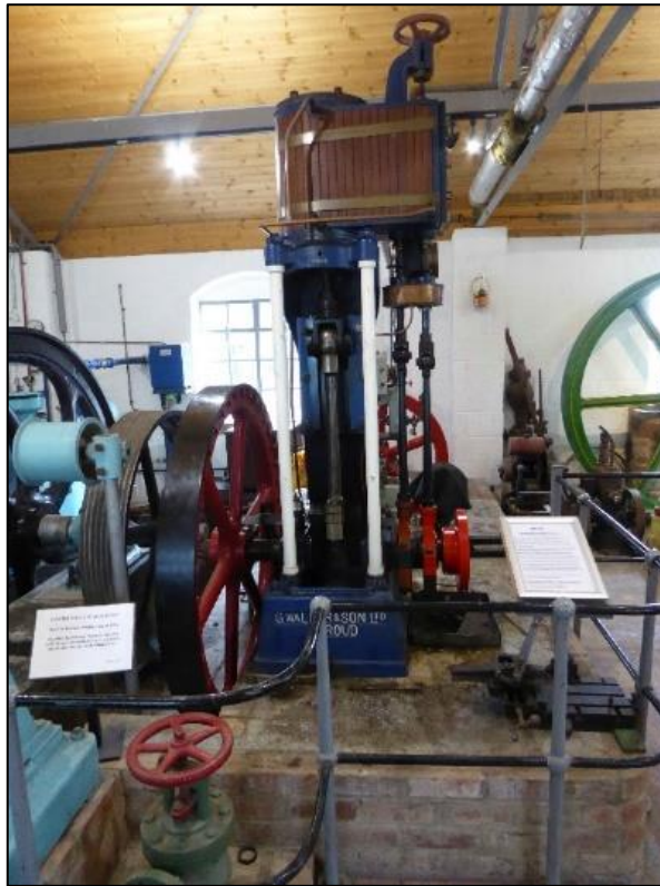
Fig 4. Single cylinder double-acting steam engine, G Waller & Sons, Phoenix Iron Works, Stroud. Ex Poole gas works exhaustor plant
