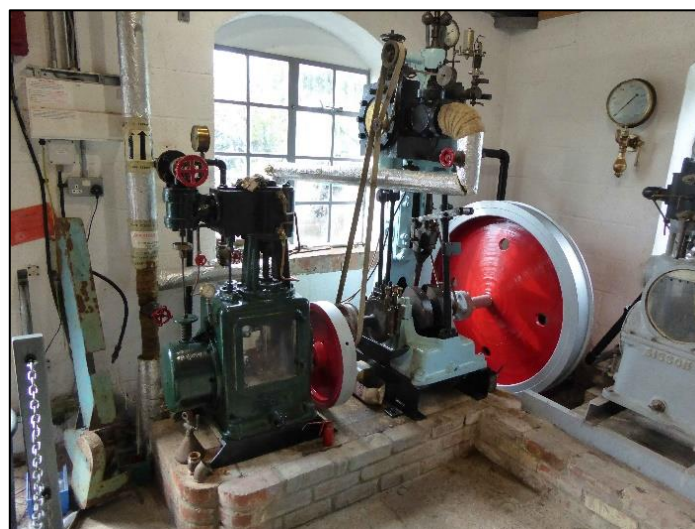
Fig 3. Sissons experimental double-acting steam engine
