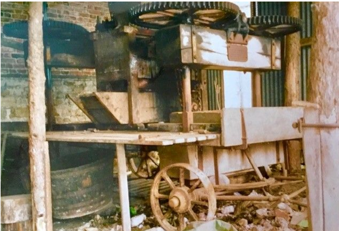
A rather dilapidated Workmans portable combined mill and press. This was up for sale on a Slimbridge farm around a decade ago (courtesy Ian Standing)
