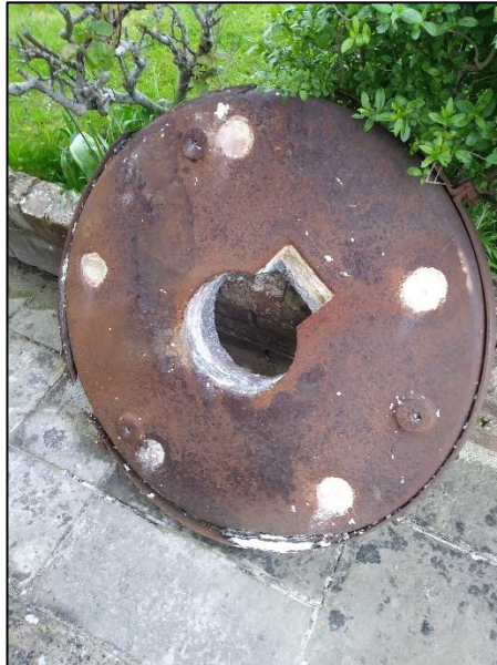
Figure 6 The heavy iron back of a composition stone. This is a bedstone – note the three lugs that carried adjustment screws
