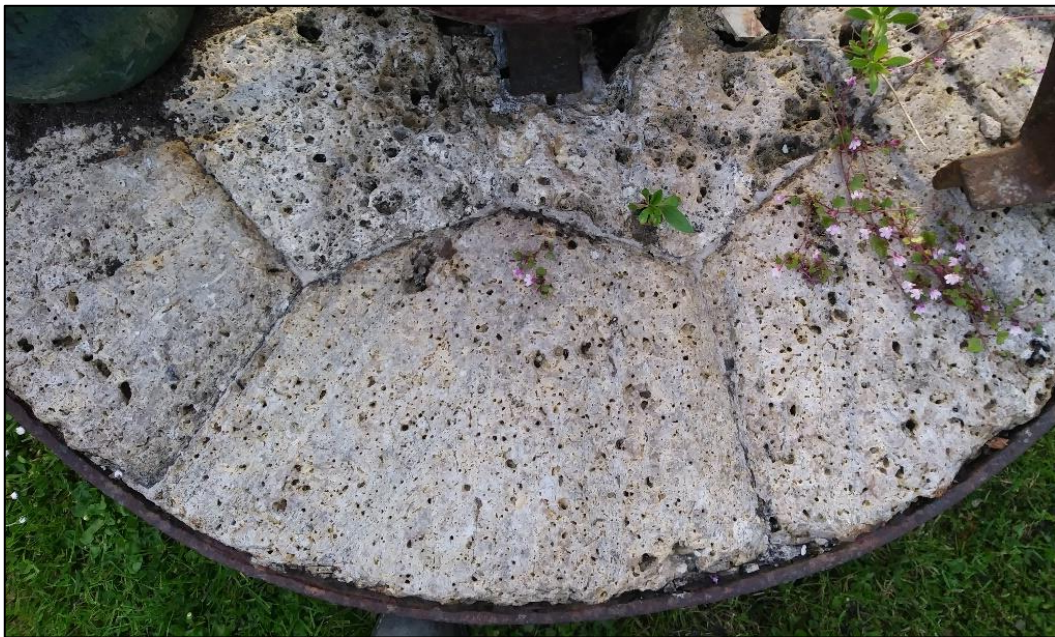
Figure 1 A typical French burrstone – note the individually shaped segments
